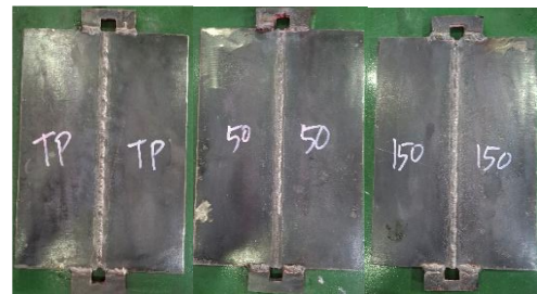
Gambar 3. Hasil pengelasan ( root pass )
