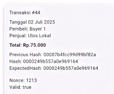
Figure 6. Transaction Information Stored in a Single Blockchain Block
