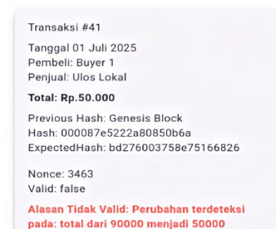
Figure 8. Transaction Information of the Manipulated Block
