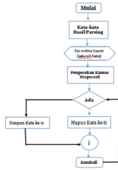
Figure 5. Flow diagram Filter Stopword Removal
