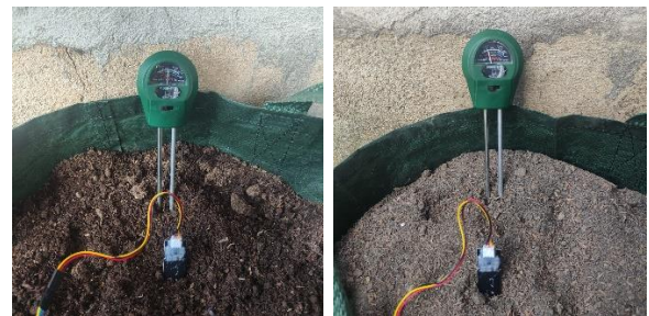
Figure 10. Testing and measuring the soil moisture sensor readings for dry and moist soil.
