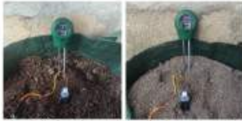
Figure 9. Testing and measuring the soil moisture sensor readings for dry and moist soil.
