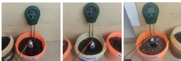
Figure 11. Testing and Data Collection of Soil Moisture Sensor Values
