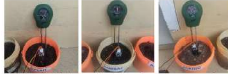
Figure 10. Testing and obtaining soil moisture sensor values.
