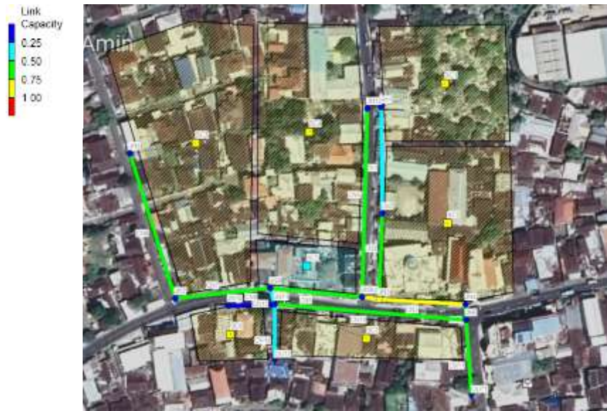
Figure 3. Overflowing channels identified by EPA SWMM 5.2 in Bastiong Karance area
