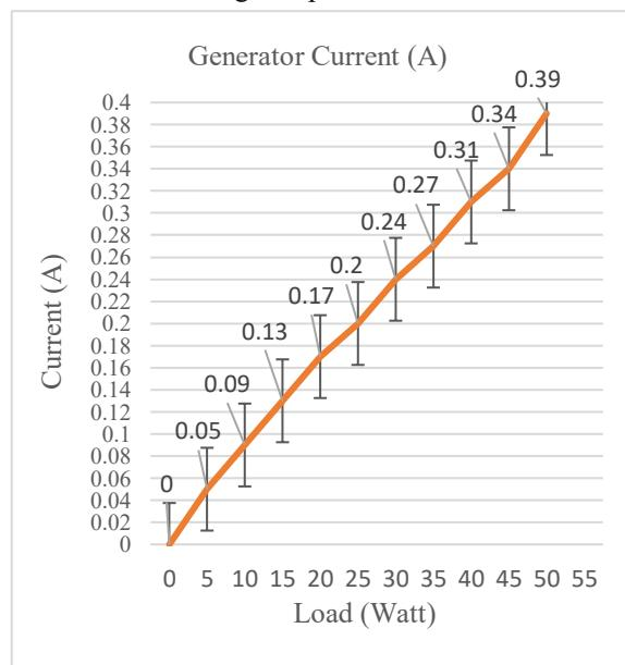
Figure 16. Graph of Inverter Output Current Measurement Results
