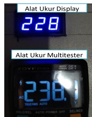
Figure 13. Inverter Output Volyage
