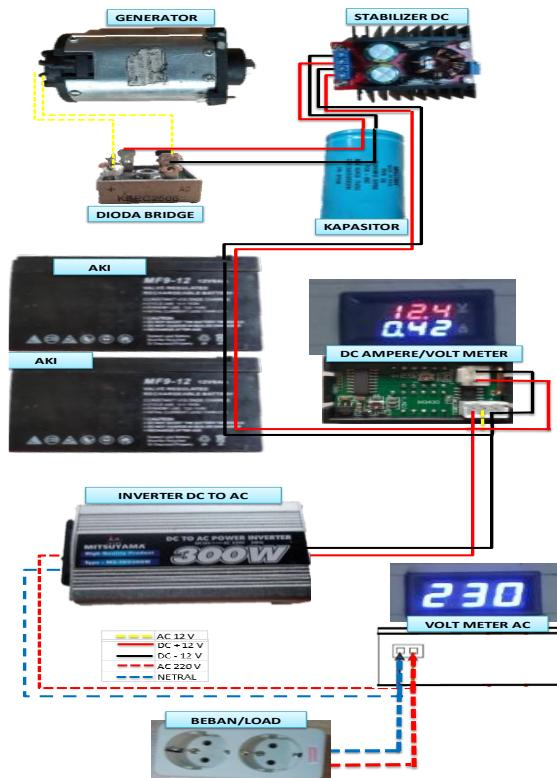
Figure 3. Wiring Diagram
