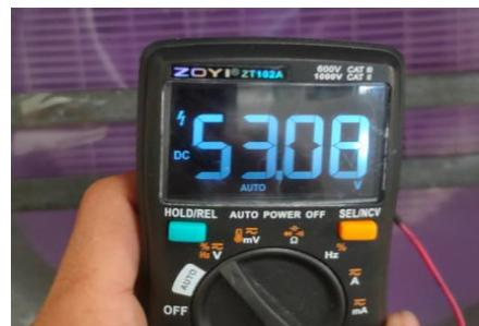
Figure 9. Generator Voltage Output Measured
