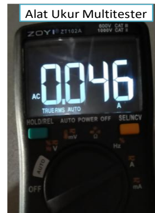
Figure 15. Digital Multimeter Display for Inverter Output Current Measurement
