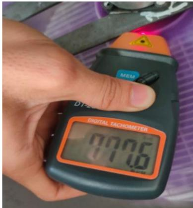
Figure 7. Generator Rotational Speed
