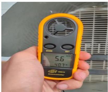
Figure 5. Wind Speed Measurement
