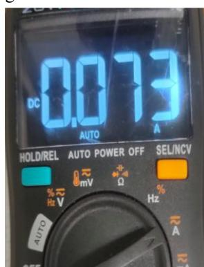
Figure 11 . Generator Current Output Measured
