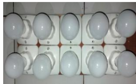
Figure 4. Load Test with Lighting Units
