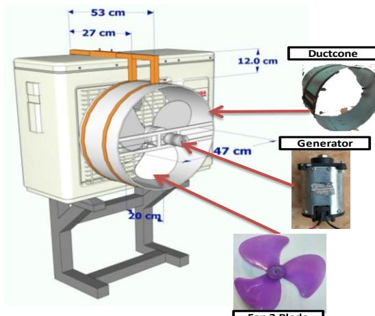
Figure 2. Mechanical Design
