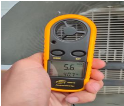
Figure 5. Wind Speed Measurement
