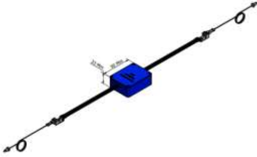
Figure 4. IoT-based K-type thermocouple
