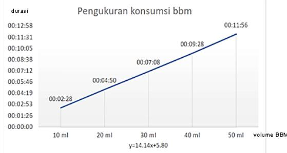
Figure 4. Duration vs volume graphic during idling condition test
