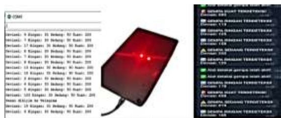
Figure 4. Serial Monitor Display and Telegram Notification When Moderate Vibration Occurs
