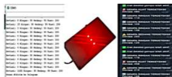
Figure 5. Serial Monitor Display and Telegram Notification When Strong Vibration Occurs
