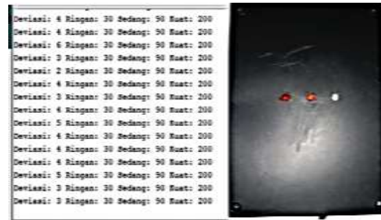
Figure 2. Serial Monitoring Display and Physical Form of the Device When There is No Vibration
