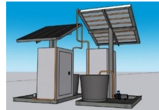
Figure 3. 3D prototype design of copper pipe cooling layout on PV panel
