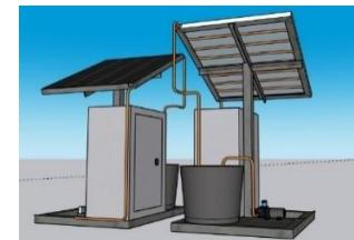
Figure 3. 3D prototype design of copper pipe cooling layout on PV panel
