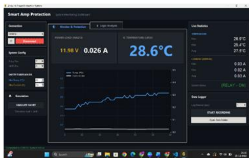
Figure 6. Python-based monitoring and protection dashboard interface.
