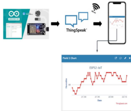
Figure 3. Software programming scheme for measuring carbon monoxide (CO) levels
