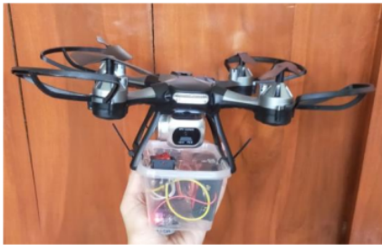
Figure 5. CO level measuring device using drone
