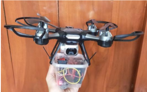
Figure 5. CO level measuring device using drone
