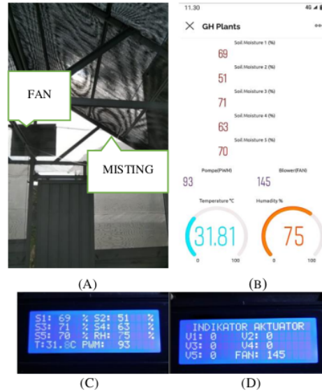
Figure 16. (A).Installation of output devices in the greenhouse, (B).Monitoring results through the bynk application, (C) and (D) Monitoring results through the actuator incubator
