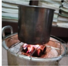
Figure 5. Briquette Testing Using Biomass Stove
