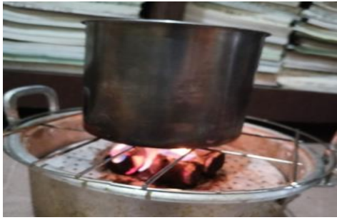
Figure 5. Briquette Testing Using Biomass Stove
