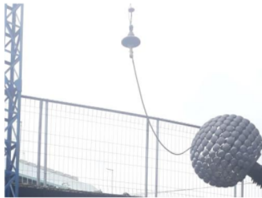
Figure 4. Insulator Flashover Testing
