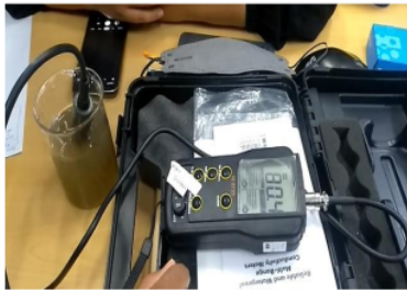
Figure 5. ESDD and NSDD Measurement
