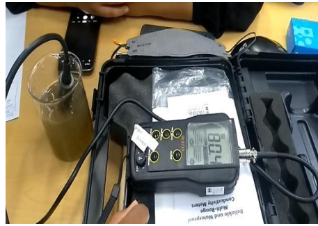
Figure 5. ESDD and NSDD Measurement
