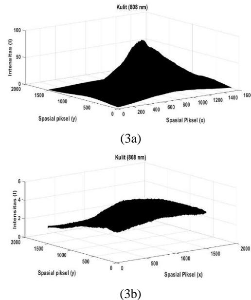
Figure 3. Infrared Ray Intensity (3a) condition without substance (b) substance with a thickness of 0.4 cm
