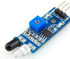
Figure 3. Infrared Proximity Sensor
