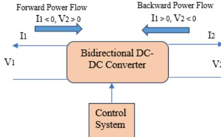
Figure 1. The general structure of bidirectional DC-DC converters
