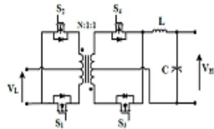
Figure 14. Flyback bidirectional DC-DC converter
