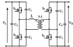
Figure 17. Dual half bridge bidirectional DC-DC converter
