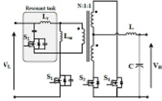
Figure 15. Forward bidirectional DC-DC converter
