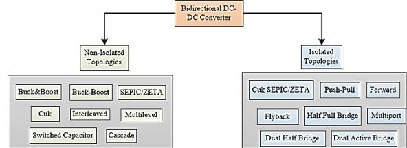
Figure 3. The classification of bidirectional DC-DC converters
