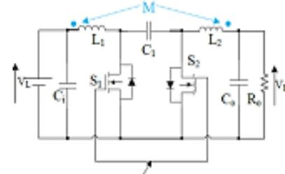
Figure 6. Cuk derived bidirectional DC-DC converter
