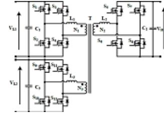
Figure 19. Multiport dual active bus bidirectional DC-DC converter
