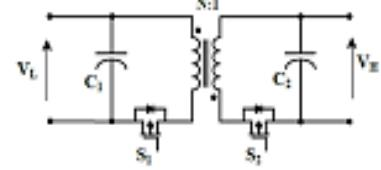
Figure 12. Isolated flyback bidirectional DC-DC converter
