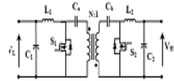
Figure 13. Isolated cuk and sepic/zeta bidirectional DC-DC converter
