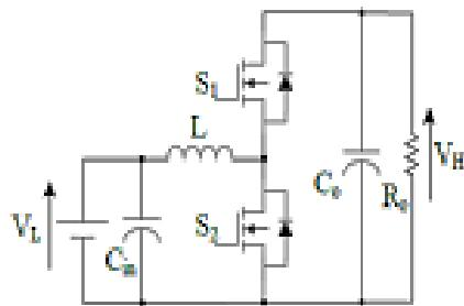
Figure 4. Buck and boost derived bidirectional DC-DC converter
