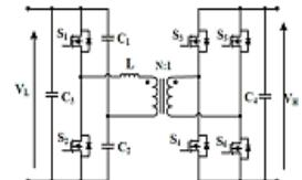
Figure 18. Half bridge and full bridge bidirectional DC-DC converter
