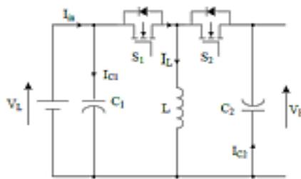
Figure 5. Buck-boost derived bidirectional DC-DC converter
