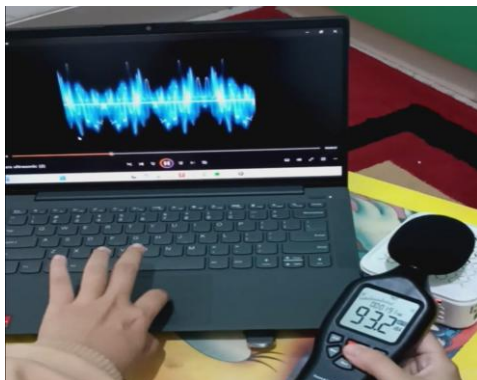
Figure 6 Decibel Measurement Process Using A Sound Level Meter
