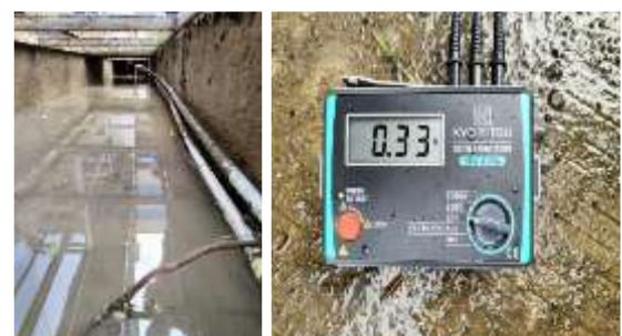
Figure 7. The results of measuring the grounding resistance of the ground rod at point A
