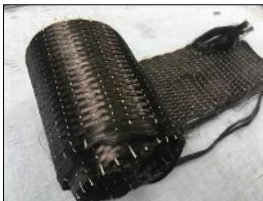
Gambar 1. Carbon Fiber Reinforced Polymer (CFRP)
