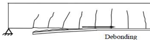
d. FRP debonding from laminate end
