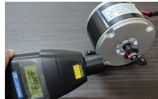
Figure 18. Measurement results of speed at 100% duty cycle
