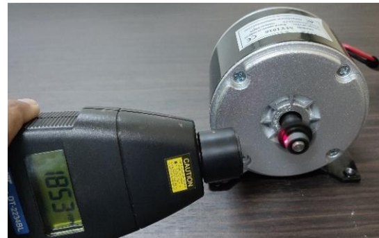
Figure 17. Measurement results of speed at 25% duty cycle
